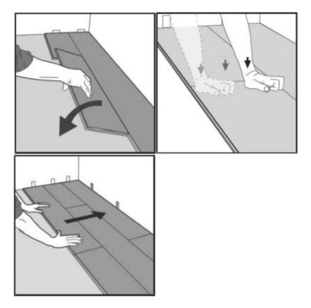
**Disassembly Guide:** Definitive Hybrid Flooring can be disassembled and reassembled if necessary as long as the flooring is not damaged. Disassemble the planks by sliding horizontally as shown in diagrams below.
