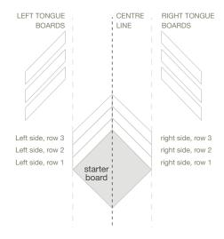
Set the right-tongue plank to the right-hand side of the starter board with the grooved side snug to the starter board and the tongue side facing out to towards the room, make sure the upper end is engaged with that of the left-tongue plank and the top side of plank be exactly in line with the centre line, press the right-tongue board down with to the sub-floor over the moisture barrier membrane.
