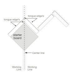
Set the right-tongue plank to the right-hand side of the starter board with the grooved side snug to the starter board and the tongue side facing out to towards the room, make sure the upper end butt is engaged with that of the left-tongue plank and the tongue end of the right-tongue plank lines up with the tongue side of the left-tongue plank, press the right-tongue board down with to the subfloor over the moisture barrier membrane.
